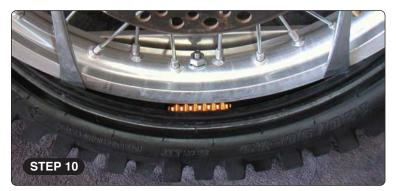
1 Conce the rim is **COMPLETELY** inside the tire, use the tire irons to start pulling the beads back onto the rim. **IMPORTANT**: Always start <u>opposite</u> the rim lock and **FINISH** pulling the last of the tire bead onto the rim at the rim lock location. Flip the wheel over and repeat the same procedure again. **FINISH** pulling the last of the tire bead onto the rim at the rim lock location.
