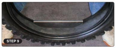
1 Orim inside the tire against the Guide Plate and **keep** downward pressure on the rim while using tire irons to pull the bead open. Keep pushing downward on the rim until the rim is completely inside the tire. Remove the guide plate.
